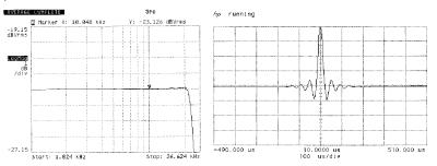
Frequency response and transient characteristics of the short FIR filter
