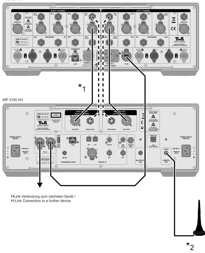
$<sup>\</sup>ensuremath{^{*1}}$  If both types of connection are present on the amplifier , we recommend the symmetrical option
