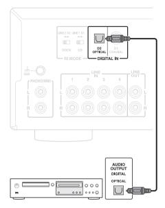
When playing back, turn the INPUT selector and light up the input source LED corresponding to the connected terminal. (Example: "D 2" when connected to the OPTICAL (D2) terminal)
