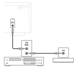
When there are two RI terminals on the equipment, one can be connected to this unit and the other can be connected to other equipment, allowing to link both equipment to this unit. Similarly, it is possible to increase the equipment to be linked. There is no specification for order to connect the equipment.
