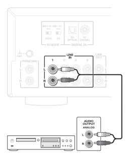
When playing back, turn the INPUT selector and light up the input source LED corresponding to the connected terminal. (Example: "LINE 1" when connected to the LINE IN 1 terminal)
