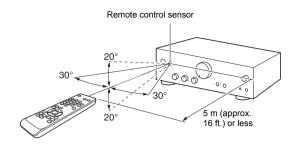
When using the remote control, point it toward the remote control sensor on the unit from a distance of 5 m (approx. 16 ft.) or less.
