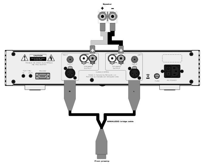
Figure 3: Bridged-Mono operation of the Neo 330A Power Amplifier
